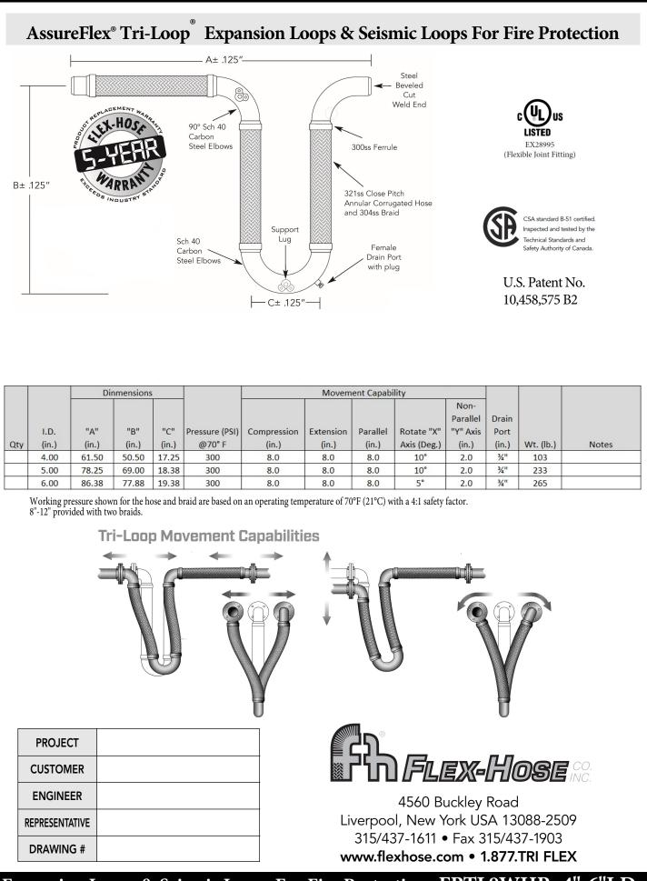
Expansion Loops & Seismic Loops For Fire Protection FPTL8WHP 4"-6"I.D.
