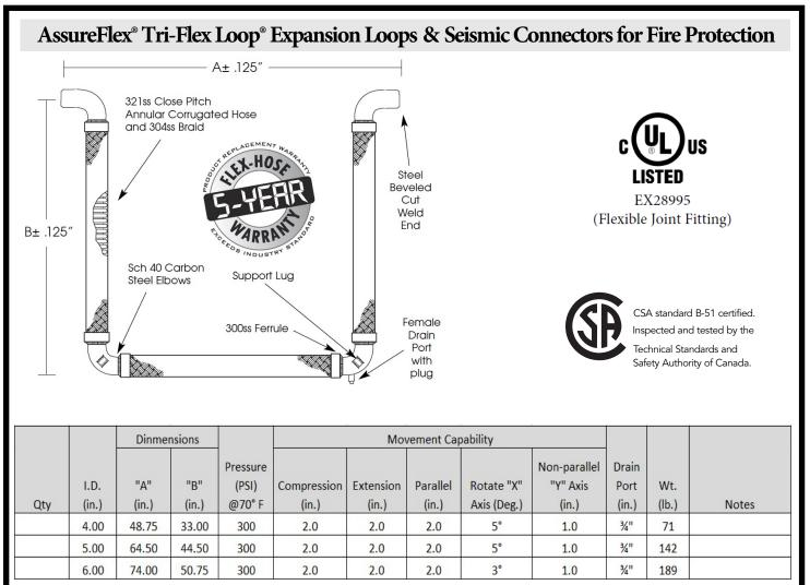
Working pressures shown for the hose and braid are based on an operating temperature of  $70^{\circ}F(21^{\circ}C)$  with a 4:1 safety factor. Provided with two braids.
