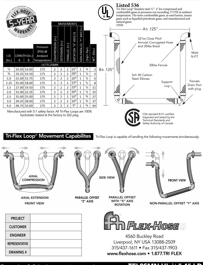
Expansion & Seismic Loops UL536 Listed
